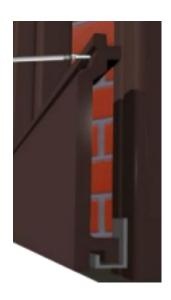
You will need to pre-drill a pilot hole into the composite joist and attach the starter clip using a screw that is at least 15mmlong.
